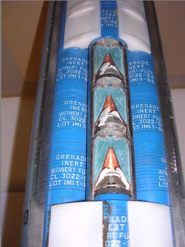
Inert M85 submunitions inside a model of a M395 155mm artillery projectile on exhibit at the Seminar on Technical Preventative Measures, Thun, Switzerland, May 2004. © 2004 Human Rights Watch
